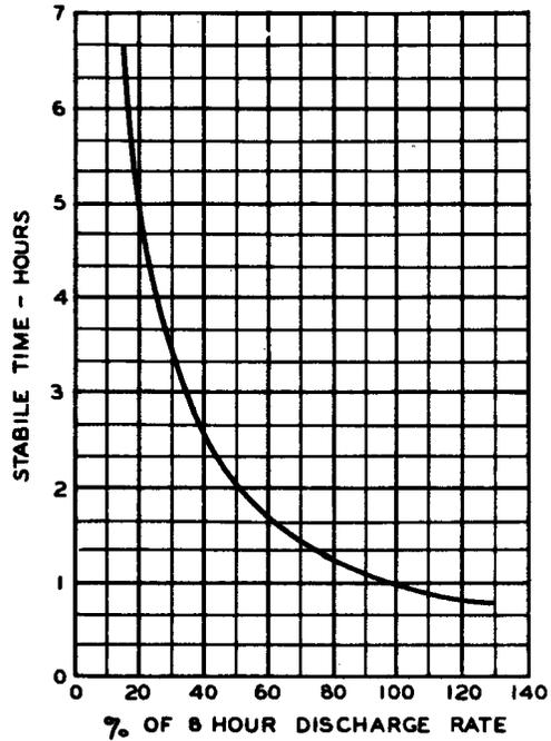
Fig. 2 - Constant Current Equalizing Charge
