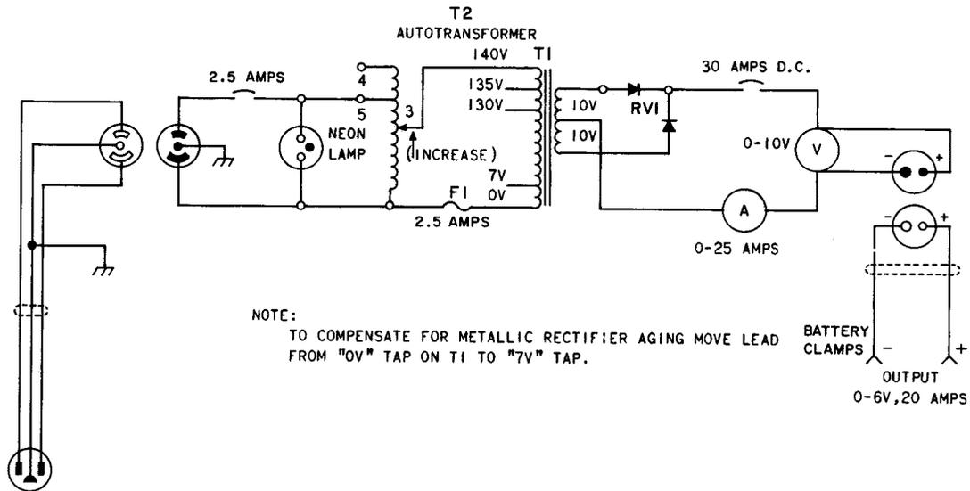
Fig. 5—KS-15687 L3 and L4 Rectifiers—Schematic
