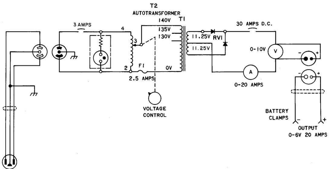
Fig. 4—KS-15687 L1 and L2 Rectifiers—Schematic
