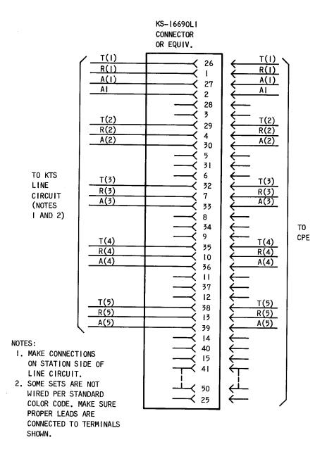
Fig. 5—Connections for USOC RJ24X—Multiple Bridged Tip and Ring With "A" Lead Control, Standard Appearance
