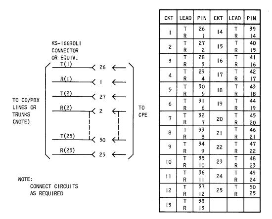
Fig. 2—Connections for USOC RJ21X—Multiple Bridged Tip and Ring
