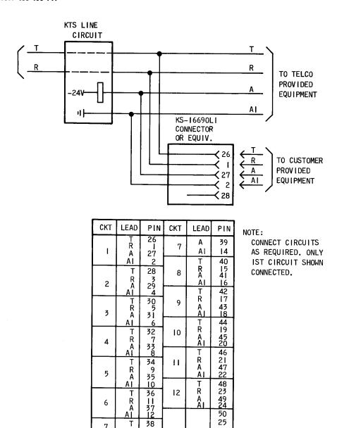
Fig. 4—Connections for USOC RJ23X—Multiple Bridged Tip and Ring Behind Line Circuit With "A" Lead Control
