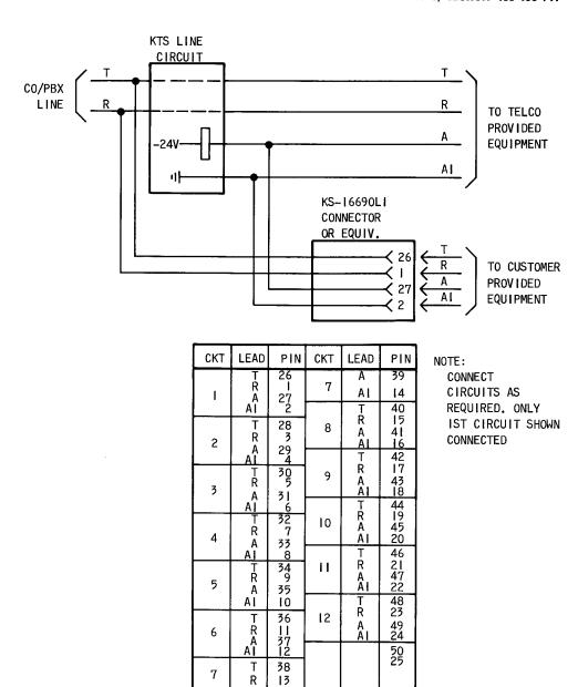
Fig. 3—Connections for USOC RJ22X—Multiple Bridged Tip and Ring Ahead of Line Circuit With "A" Lead Control
