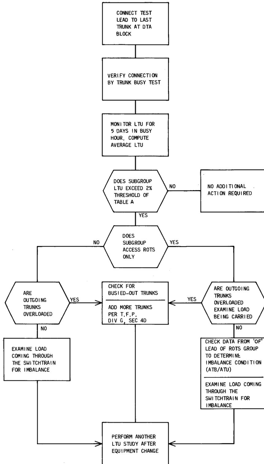
Fig. 5—SXS Subgroup LTU Quick-Test Procedure
