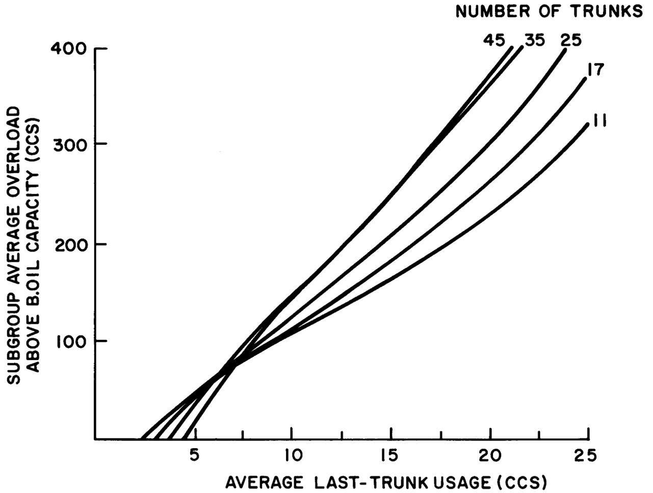
Fig. 2—Subgroup Average Overload Versus Average Last-Trunk Usage for Different Graded Multiple Configurations (Non-ROTS Accessing) with *Low* Day-to-Day Variation in Offered Load
