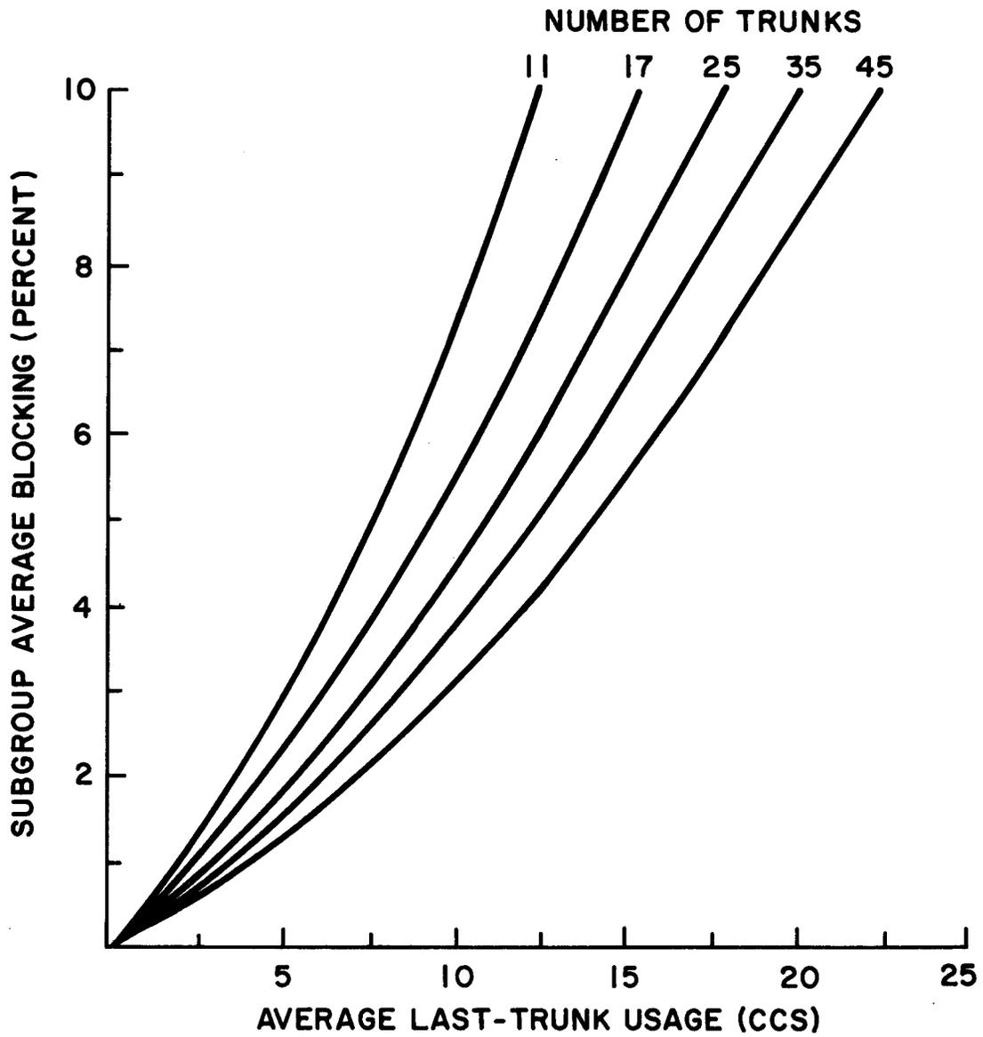
Fig. 1—Subgroup Average Blocking (Percent) Versus Average Last-Trunk Usage for 11, 17, 25, 35, and 45—Trunk Gradings with *Low* Day-to-Day Variation in Offered Load
